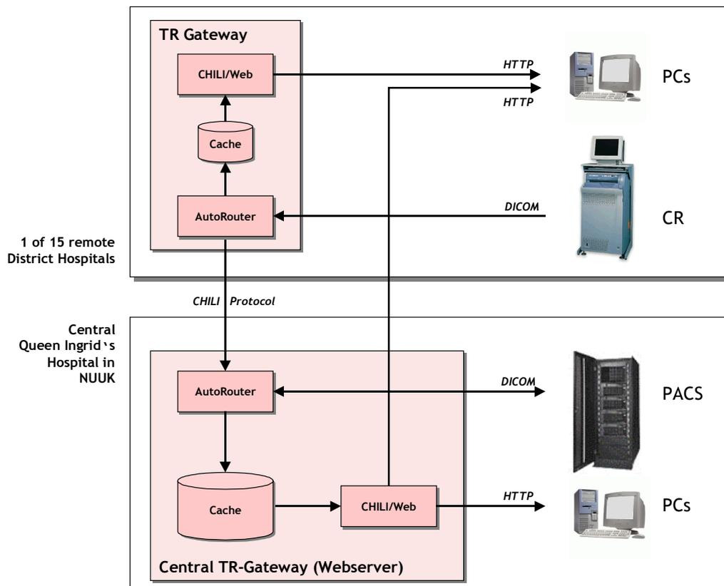
Fig. 1. (Simplified) data flow and architecture of the central and remote TR-Gateways
