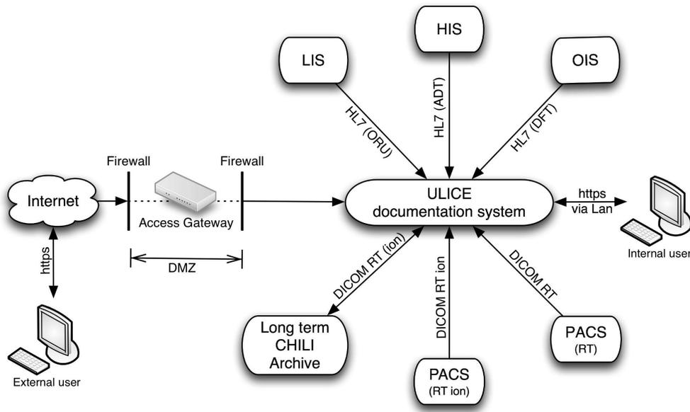
Figure 2. Connected systems and used protocols
